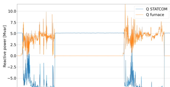
Figure 8 Furnace and STATCOM module reactive powers during furnace operation. The reactive power of the furnace (orange) fluctuates rapidly and unpredictably, but Merus® STATCOM (blue) can react almost instantly and control its' reactive power output as needed.
